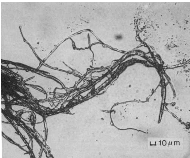
Fig. 6. Optical micrograph of LDPE fibers formed at \dot{\gamma} = 84 s^{-1} using a capillary with D/d = 5 and \alpha = 15^\circ . The blend is 70/30 Wanin SR/LDPE.
